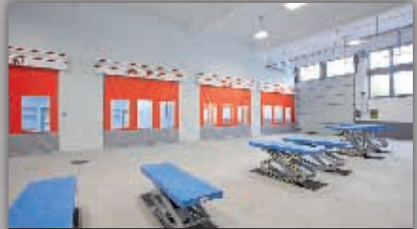
SERIE PREP STATION CON TENDA MOTORIZZATA SERIES OF PREP STATIONS WITH MOTORIZED CURTAINS
